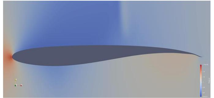
Fig 3: Optimized shape with diffusion constraint.  $Cl = 0.50$ ,  $t = 0.105$ ,  $Cd = 0.038$
